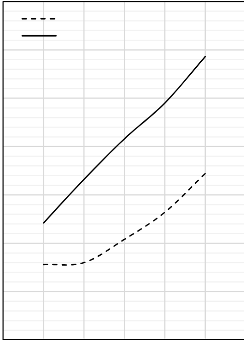
Fig. 5 Switching loss vs. gate resistor
